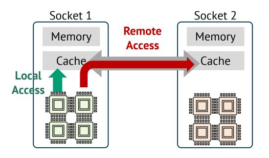
Accessing local socket memory is faster than remote socket memory
