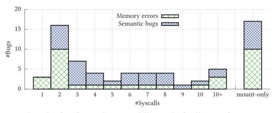
Fig. 14. The number of syscalls required to trigger each file system bug found by HYDRA after minimization.
