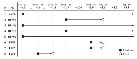
Fig. 19. Lifespan of crash consistency bugs in stable Linux kernel, from v4.1 to v5.3. The black dot ( $\bullet$ ) denotes the version in which bug is introduced, the white dot ( $\bigcirc$ ) marks the version in which bug is fixed, and the arrow ( $\rightarrow$ ) refers to the affected versions. Note that the bug ids (#) are consistent with those of Table 6.
