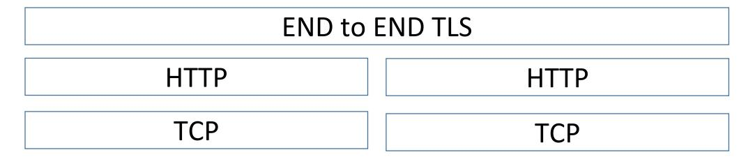
Secure split connection at edge using SGX
